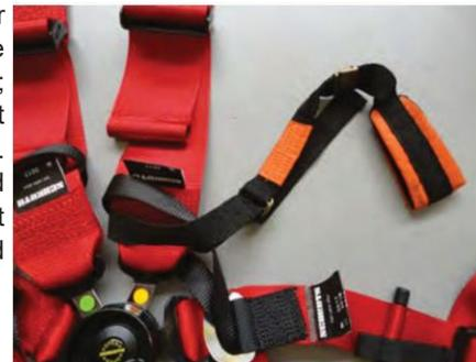
In an open car like the Saker Sniper and the Saker Sprint, two arm restraints must be worn. The arm restraints are attached to the right and left shoulder belt.
