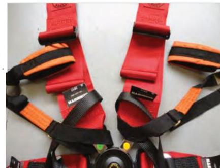
**Important!** Make sure the arm restraints are completely released with releasing the seat belts.
